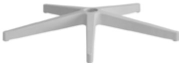
5 star light grey nylon base \varnothing 700 mm, high resistance with reinforcing steel ring.
